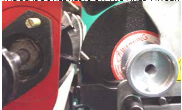
FIG. 75 THE MOVEABLE INDEXING FINGER SPRINGS FORWARD TO BE IN FRONT OF THE BLADE.
