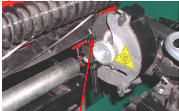
FIG. 75 THE MOVEABLE INDEXING FINGER SPRINGS FORWARD TO BE IN FRONT OF THE BLADE.
