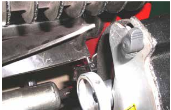
FIG. 76 THE MOVEABLE INDEXING FINGER WILL BE IN FRONT OF THE BLADE WHEN TRAVELING LEFT TO RIGHT.
